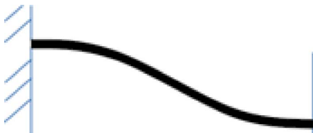
Fig. 10 Deformed flexure blade
