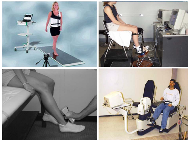
Fig. 1 Gait pressure device (top left), [6] Rutgers ankle interface (top right), [8] hand-held dynamometer (bottom left), [10] and isokinetic dynamometer (bottom right) [12]
