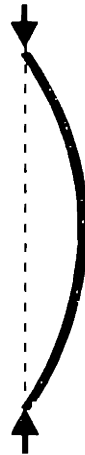
Figure 1.1: Shape of the first mode of a column with pinned ends. The shape of a column can be expressed as a combination of mode shapes. For small deflections, the modes are independent of one another, each moving at its own characteristic frequency. From a structural engineering point of view, the first mode is the most important, since buckling in the first mode occurs at a smaller load than does buckling in higher modes. The particular shape of the modes depends on how the column is supported and on the material and geometrical properties of the column
