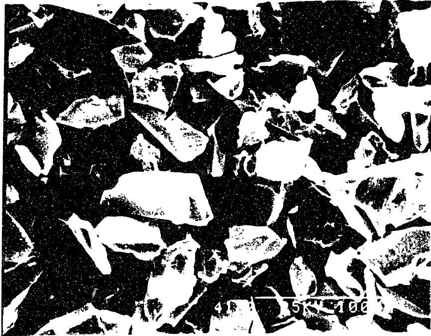
Figure 3.1 Micrograph of a typical sample of Norton 325 mesh alumina powder.
