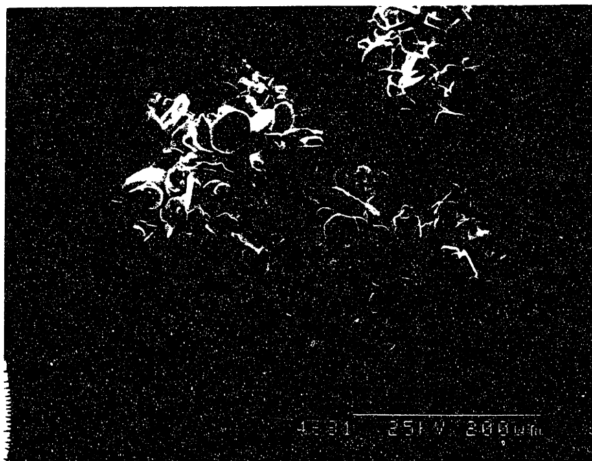
Figure 4.15 Micrograph of an 8 drop segment primitive made from Norton 30 \mu\text{m} alumina.
