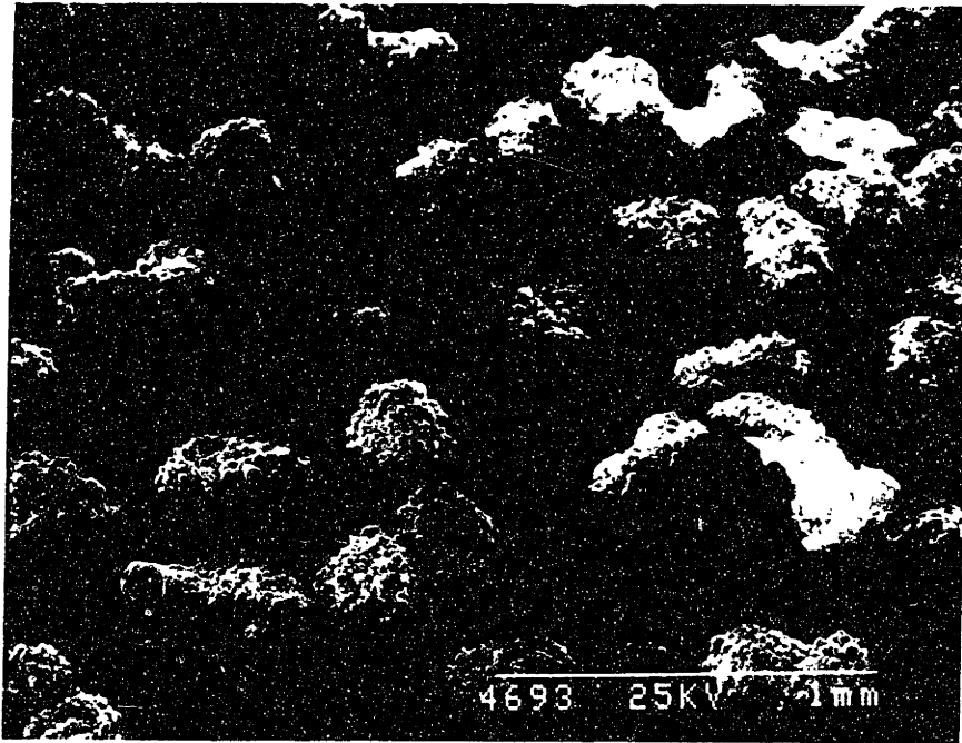
Figure 4.18 Micrograph of several spray dried 8 drop primitives.
