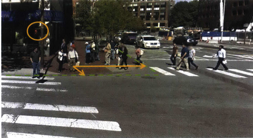
Figure 1-1: Example intersection scenario. Dotted green line denotes a rectangular approximation to the curbside in view. Orange arrows denote relative distance of a pedestrian from the two curbsides, which can indicate pedestrian intention. Pedestrian traffic light status is highlighted in orange, which also influences pedestrian movement.
