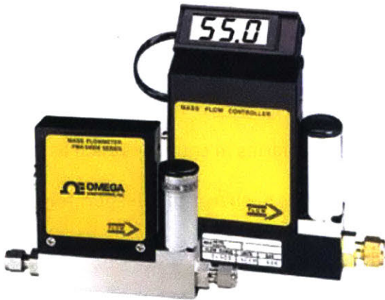
Figure 2: The image on the left is of the Omega mass flow controller used in the system. It has a D-connector on the left side of the device that allows for remote control of the gas flow setpoint and a potentiometer on the right side that can be used to input the setpoint manually. The silver cylinder on the right side is the housing for the motor that manages the opening of the control valve.
