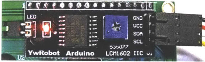
Figure 12: A close up to the microcontroller board on the back of the lcd display and shows the four wire pins, GND,Vcc, SDA and SCL .
