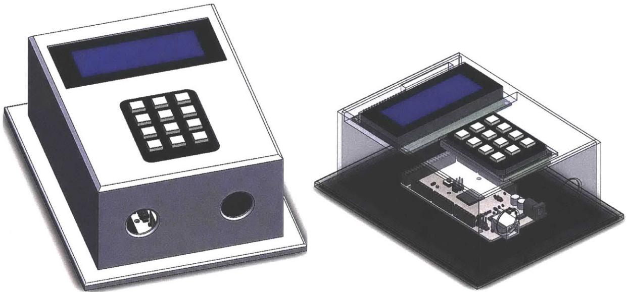
Figure 20: CAD models of a housing for the microcontroller, keypad, and lcd display.
