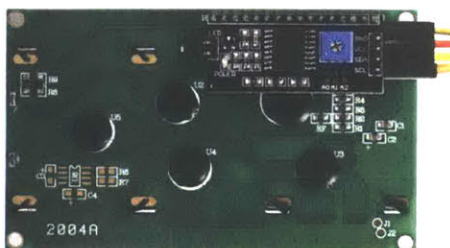
Figure 7: The back of the lcd display with the microcontroller board shown on the top right corner.
