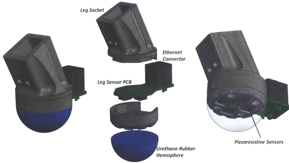
Figure 6-5: CAD representation of the robot’s soft foot sensor. The hemispherical urethane rubber contacts the ground and deforms under load. The pressure increase from this deformation is captured by an array of piezoresistive sensors. This lightweight, waterproof device can measure shear and normal forces applied to the rubber hemisphere.
