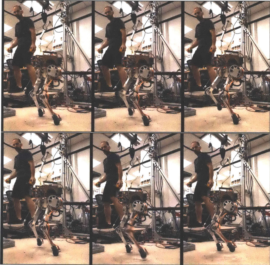
Figure 7-11: Sequence of snapshots for teleoperated stepping in place. The robot cannot statically balance during single stance, it must continually move in order to be dynamically stable.
