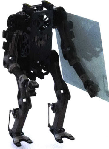
Figure 3-1: Power Plane representation of the HERMES humanoid robot left arm: the limb has six degrees of freedom but high power actuators drive only two, composing a plane. The remaining four auxiliary Degrees of Freedom are actuated by low power actuators.
