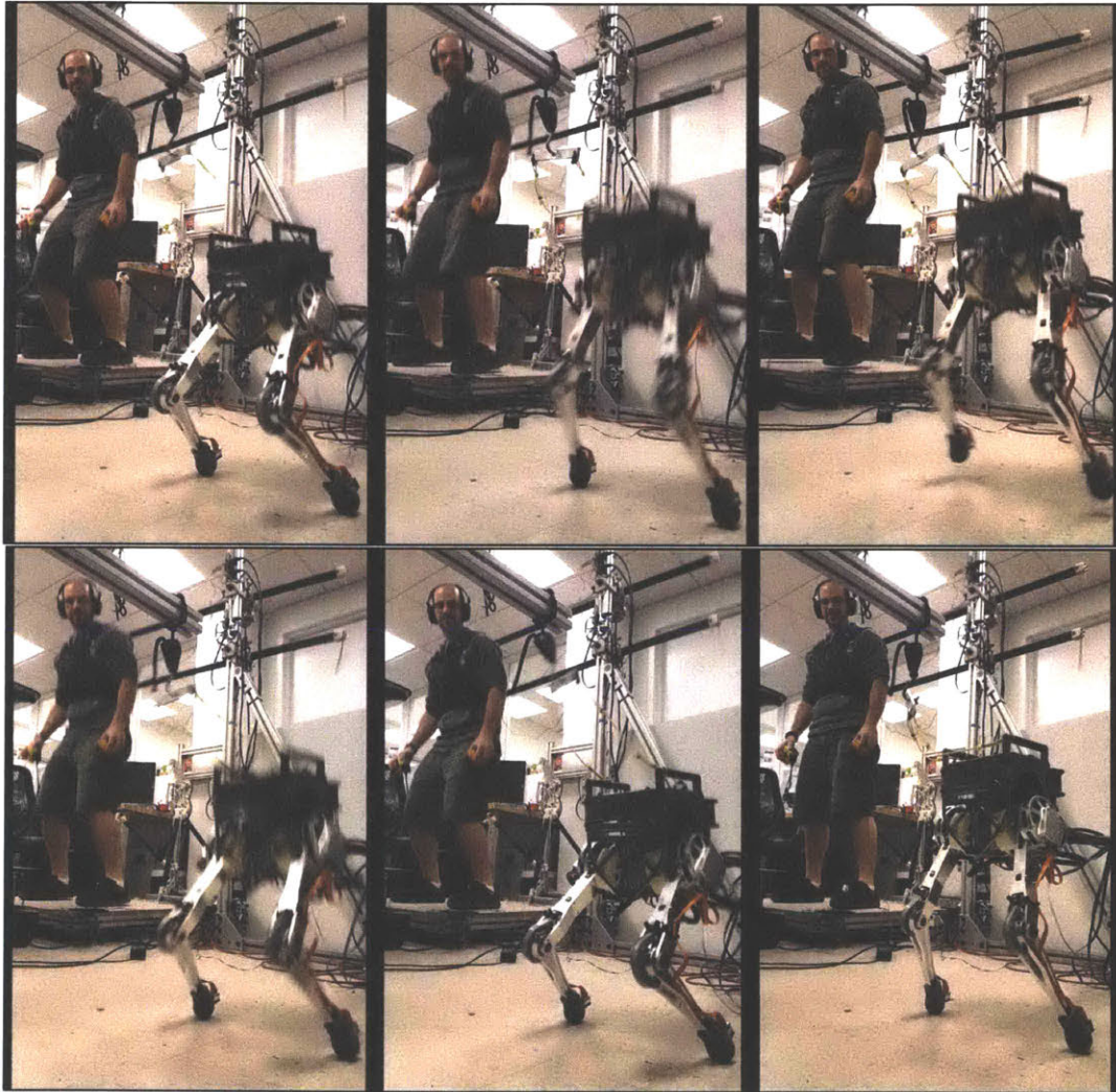
Figure 7-14: Sequence of snapshots for teleoperated dynamic jump. Notice on the top right sub-figure when the operator and the robot are both in flight.
