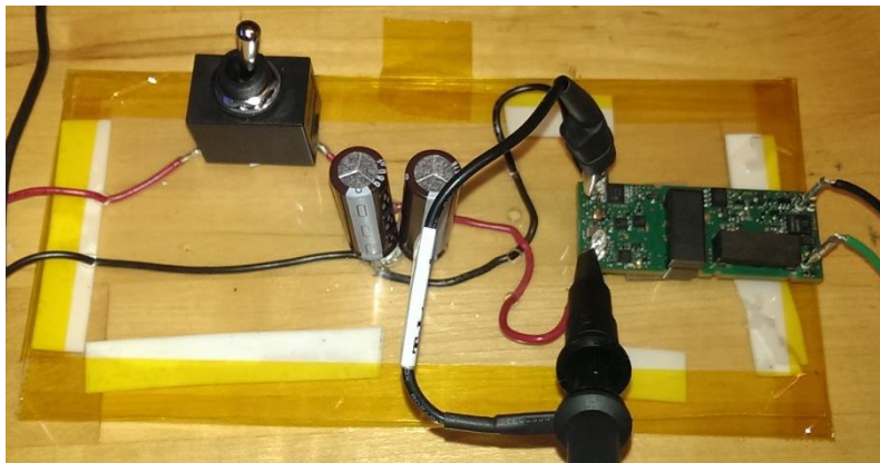
Figure 4.8. Experimental setup for testing hold-up time. The capacitance used is 2x EKYB800ELL681MK40S. The converter used is the SynQor SQ60120ETA20, which regulates its output voltage to 12 V. The capacitors are charged to an initial voltage of 72 V and the load resistor is selected as 1.2 \Omega to set the constant output power drawn to 120 W. (Note: for this early test, a nominal rated total output power of 240 W was used instead of 250 W.)
