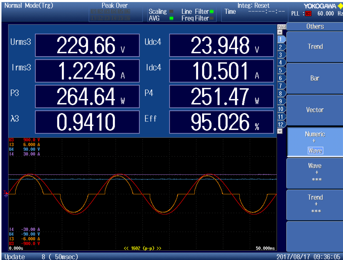
Figure 8.3. Line voltage (red), line current (yellow), output voltage (blue) and output current (purple) for the following operating point: input of 230 Vac output voltage of 24 V and output power of 251 W. The power factor is 0.941 and efficiency 95.02%. The line current is set to follow the line voltage. However the current sensor is placed after the EMI filter and thus the controller makes the stacked converter input current sinusoidal. The line current is slightly distorted by the EMI filter.
