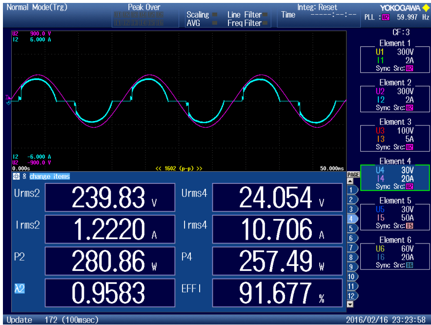
Figure 5.5. Screenshot from data measured using the Yokogawa Digital Power Analyzer. Pink: line voltage. Blue: Line current. Operating conditions: 240 V ac,rms input, 24 V dc output, 257.49 output power, 91.68% efficiency and 0.9583 power factor.
