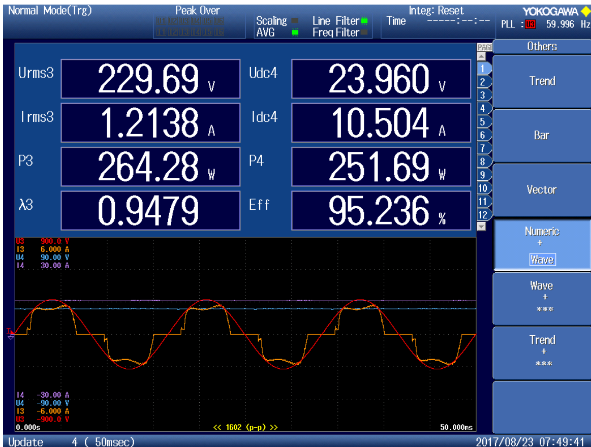
Figure 8.5. Line voltage (red), line current (yellow), output voltage (blue) and output current (purple) for the following operating point: input of 230 Vac output voltage of 24 V and output power of 251 W. The power factor is 0.948 and efficiency 95.236%. This data point is taken including all the software changes that increase efficiency. The converter does not draw peak current when the voltage is maximum.
