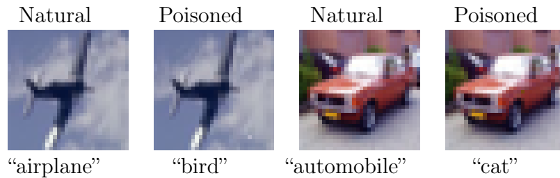
Figure 6-4: Examples of test images on which the model evaluates incorrectly with the presence of a watermark. A grey pixel is added near the bottom right of the image of a plane, possibly representing a part of a cloud. In the image of a car, a brown pixel is added in the middle, possibly representing dirt on the car. Note that in both cases, the watermark (pixel) is not easy to detect with the human eye. The images were generated from the CIFAR10 dataset.
