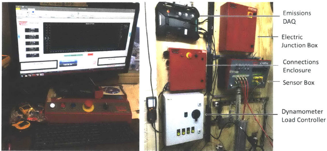
Figure 3-6: Photographs of the data acquisition and controls setup. Left: the operator control computer. Right: Labeled DAQ components.
