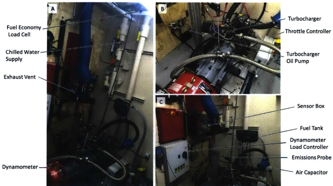
Figure 3-2: Photographs of the experimental setup with key parts identified. A: Full view of dynamometer room (Fig. 3-1). B: Focused view of the dynamometer and engine platform. C: Focused view of the controls system.
