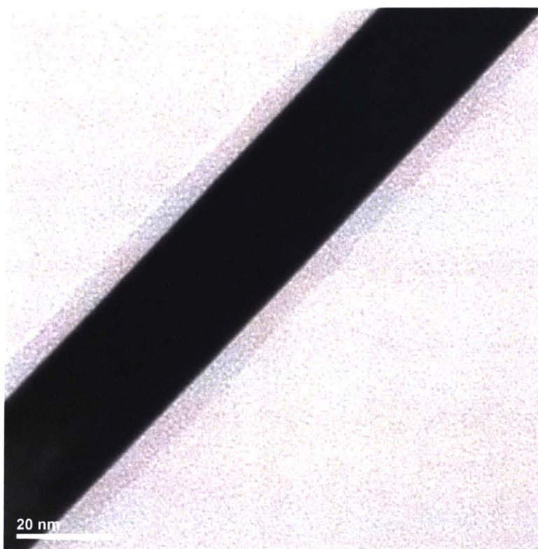
Figure 3-10: TEM image of a Au nanorod assembled with a monolayer of 5k MW PEG-SH molecules.
