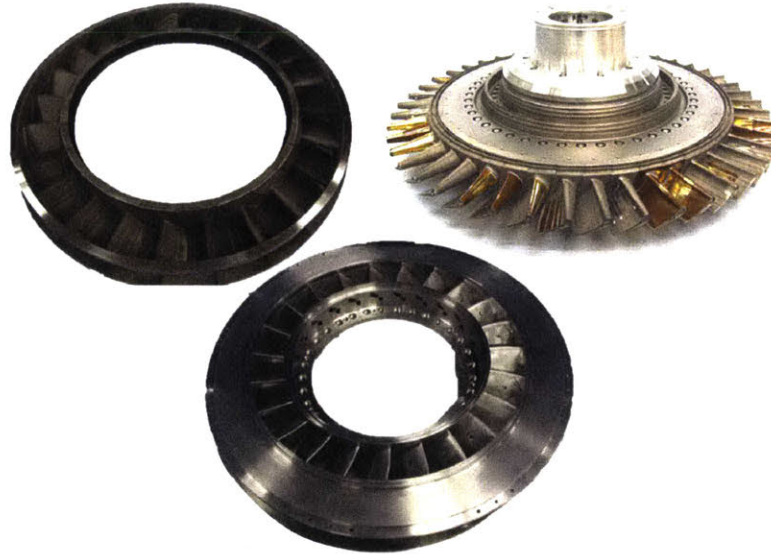
Figure 3-6: The HIT research turbine test hardware: nozzle guide vane (top left), blade wheel (top right), and downstream vane (bottom). [17]
