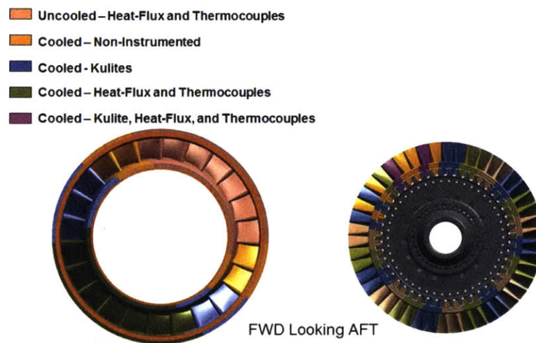
Figure 3-4: HIT turbine first vane and blade cooling schematic. The cooled airfoils are not distributed evenly around the annulus. [17]
