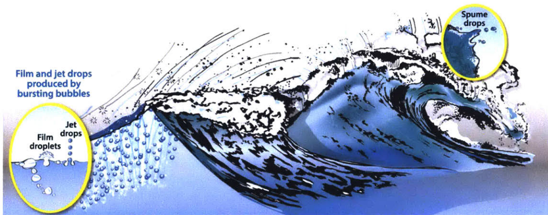
Figure 1-3: Mechanisms of generation of ocean spray, from bubble bursting (jet and film drops) to spume drops generated during wave-crest breaking. Rainfalls also contribute to bubble generation and bursting, and subsequent droplet emission [6].
