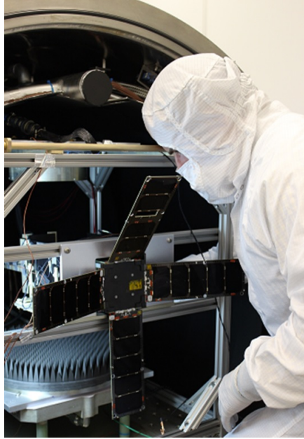
Figure 2-1: MicroMAS-1 spacecraft in a thermal vacuum chamber.[9]
