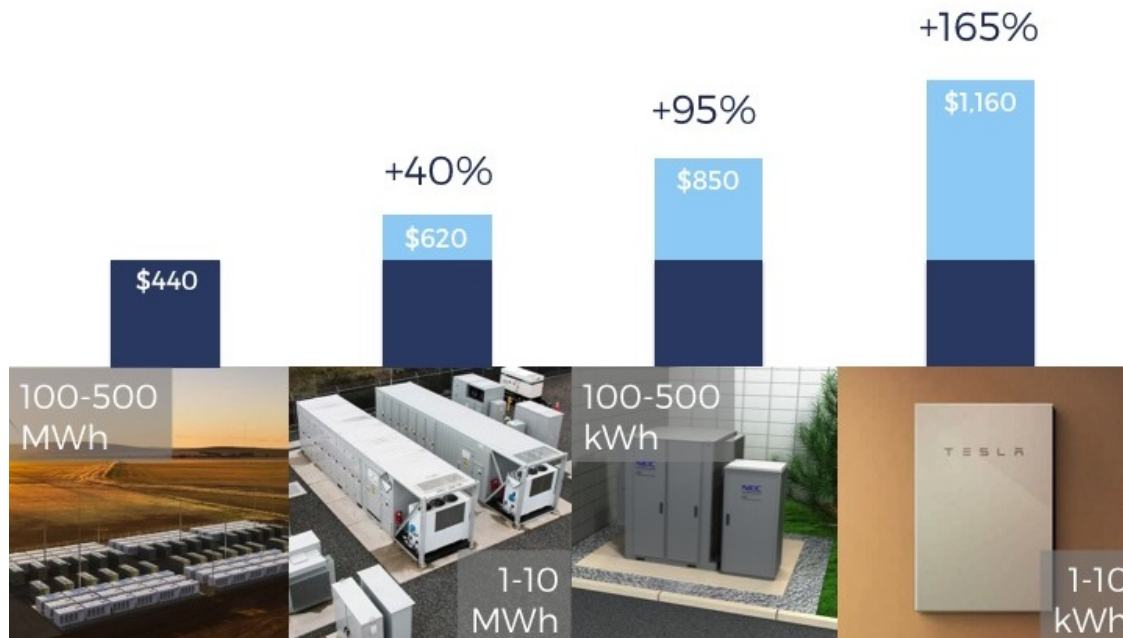
Figure 1-9: Economies of unit scale and incremental unit costs for lithium-ion battery energy storage systems (2017 costs per kWh) Data from Lazard (2017).
