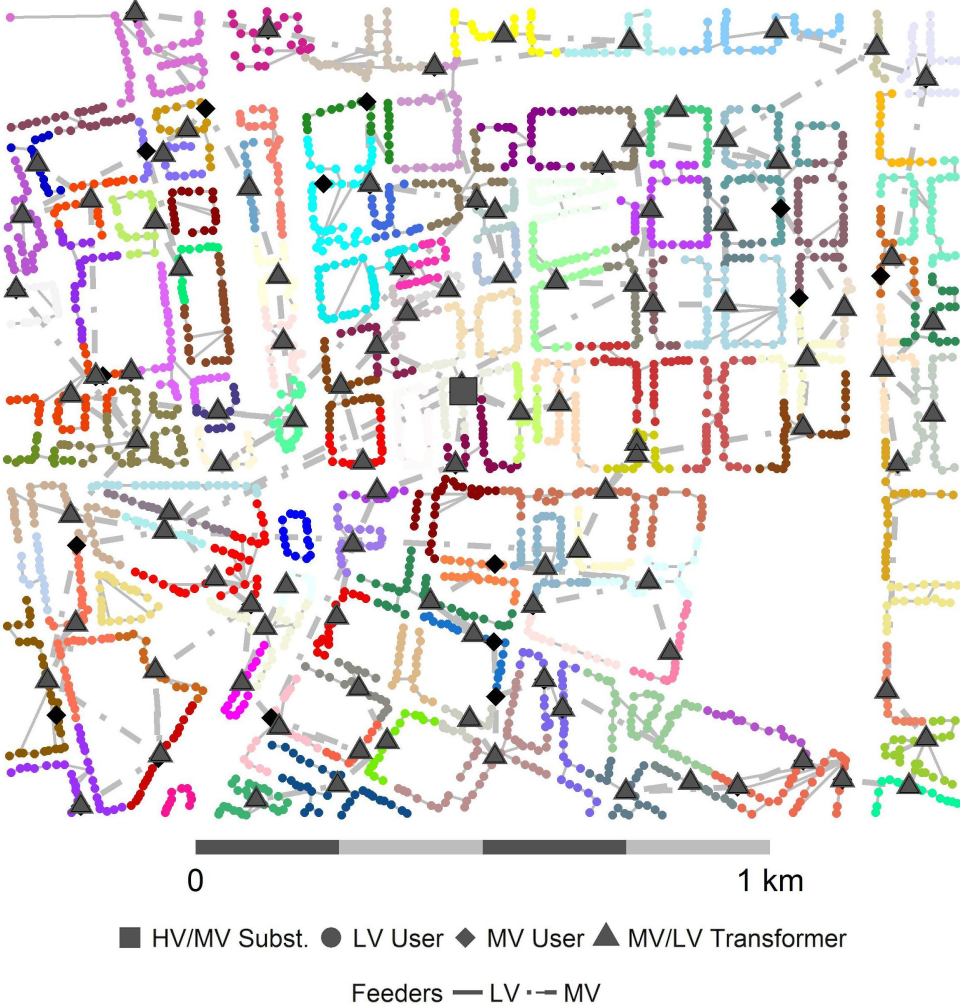
Figure 2-1: Representative urban European network map Low voltage customers are colored by network zone, where each zone corresponds to all low voltage feeders connected to a single 20 kV/0.4 kV medium to low voltage transformer. Note that line branches are depicted as vertices between any two buses. The actual line layout differs so as to adhere to street layouts and other restrictions not depicted here.
