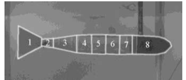
Figure 8: The fish is divided to 8 sections. The position of each segment center has been tracked photographically to find the position and orientation of each segment as a function of potentiometer voltage.
