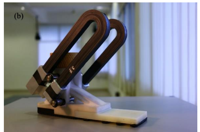
Figure 4: Solid model (a) and photograph (b) of the prosthetic foot prototype with a constant rotational stiffness at the ankle of k_{ank} = 3.7 \text{ Nm/deg} and a forefoot beam stiffness of k_{met} = 16.0 \text{ Nm}^2 .
