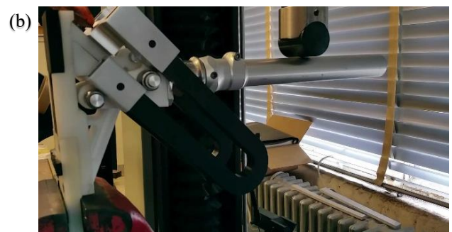
Figure 9: Experimental setup schematic (a) and photograph (b) measuring the ankle rotational stiffness k_{ankle} , with F the applied load on the shank from the Instron with the foot constrained in a vice, M the resulting moment on the ankle and \theta_{ankle} the measured ankle angle.
