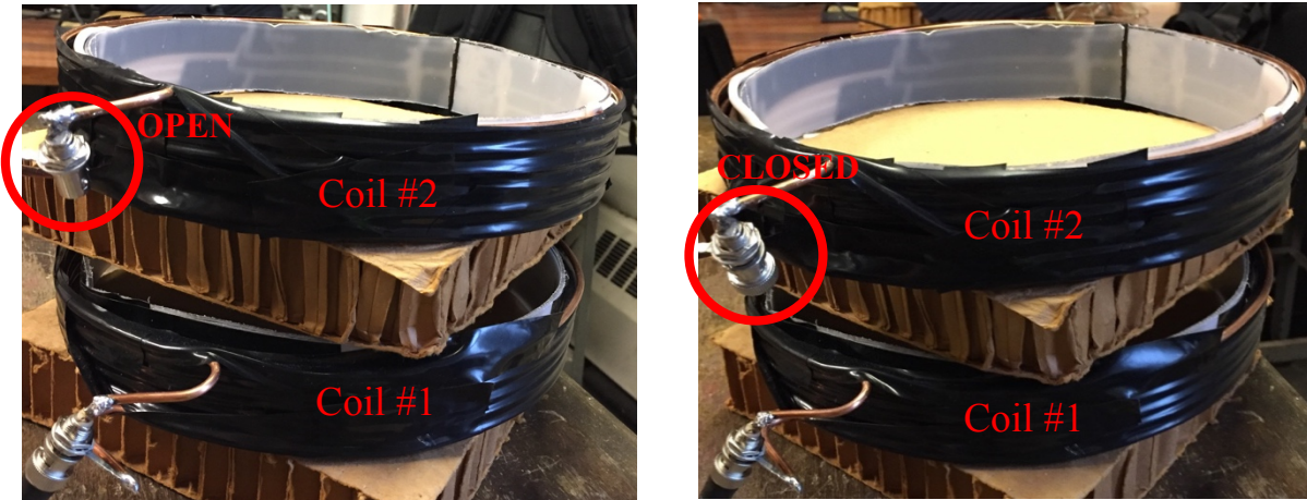
Fig. 5.3: Experimental setup for measuring the coupling coefficient between a pair of separated coils. The left image is the setup for L_1 . The right image is the setup for L_5 .
