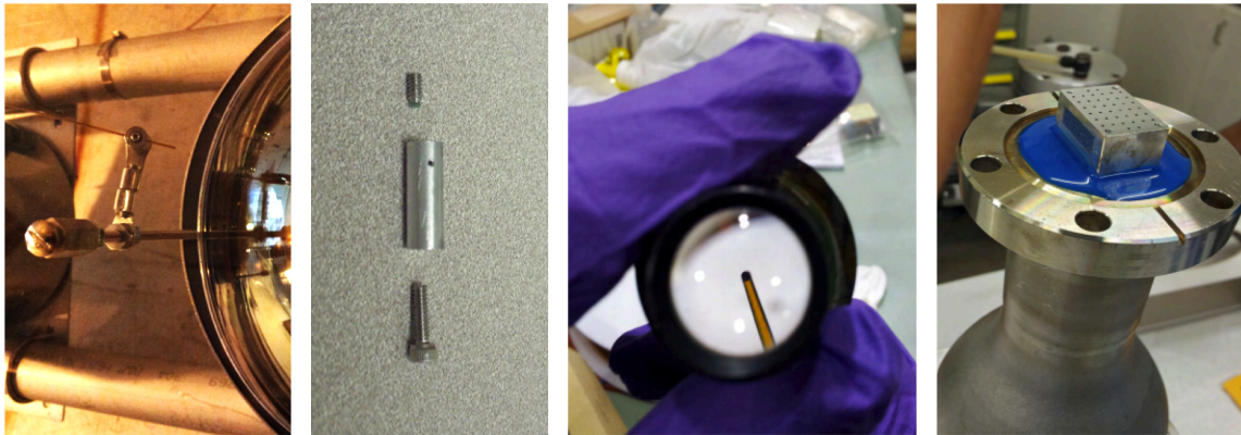
Figure 6. Left to right : the mounting stand-off which holds the fiber at each PMT ; the aluminium standoff with its nylon-tipped set-screw ; magnification of the prepared fiber end, which points towards the photocathode ; connector block being set in the custom feed-through.
