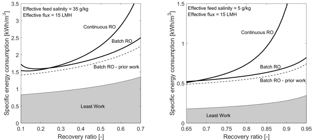
**Figure 3 and 4.** Specific energy consumption of seawater and brackish RO processes versus recovery ratio. Feed modeled as 35 g/kg and 5 g/kg NaCl solution. At an effective flux of 15 LMH, a batch SWRO plant saves energy at recovery ratios above 25% and a batch BWRO plant saves energy at recovery ratios above 67%. Prior work did not account for the disparity in operating and effective conditions (Warsinger et al., 2016). The least work of separation is shown in gray.
