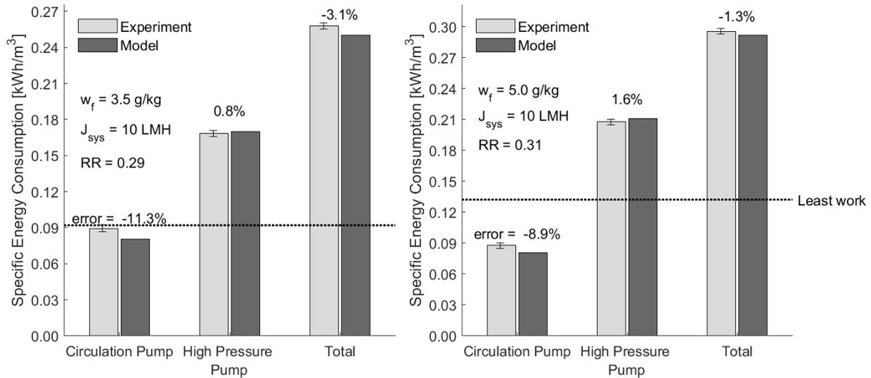
**Figure 7.** The energy consumption of the circulation pump and high pressure pump are compared to model predictions. The circulation pump operates while the system is starting up, so its work contribution is underestimated. At higher feed salinities, this error becomes smaller compared to the total work. Error bars represent 95% confidence intervals.
