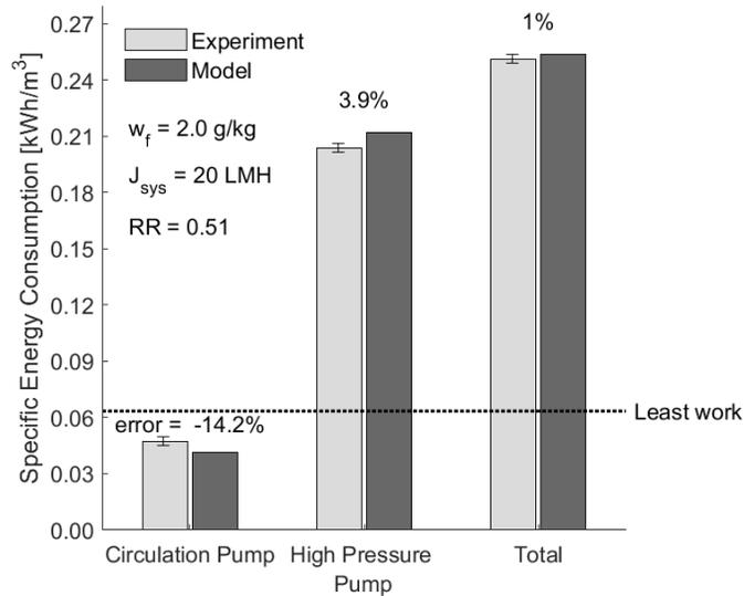
**Figure 8:** The energy consumption of the circulation pump and high pressure pump are compared to model predictions. The model overestimates high pressure pump work in part because the prototype operates at lower fluxes during system start-up. Error bars represent 95% confidence intervals.
