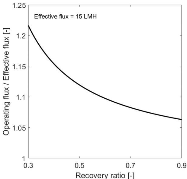
**Figure 5.** The ratio of batch operating flux to effective flux at various recovery ratios. At lower recovery ratios, the reset time accounts for a significant portion of the total cycle time so a batch system must operate at much higher flux in order to achieve the effective flux.
