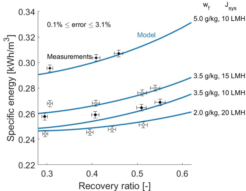
**Figure 6:** Measured and predicted specific energy consumption versus recovery ratio for various combinations of feed salinities and fluxes. The experimental results agree with the model predictions within 3.1%. Error bars represent 95% confidence intervals.
