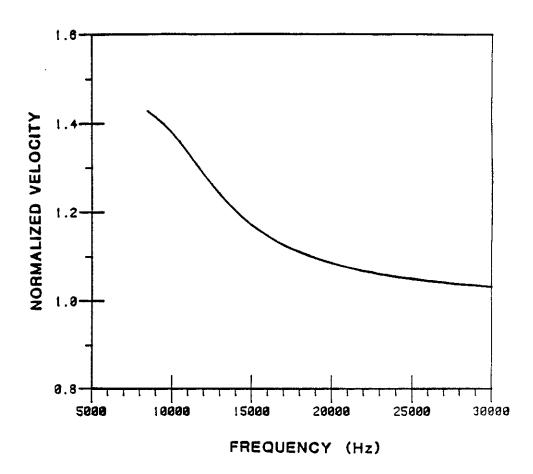
Figure 8: Pseudo-Rayleigh wave phase velocity dispersion (normalized to the borehole fluid velocity) for viscosity values of 0, 1, 10, 100, and 1000 cP
