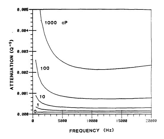
Figure 7: Stoneley wave attenuation (  $Q^{-1}$ ) for viscosity values of 0, 1, 10, 100, and 1000 cP
