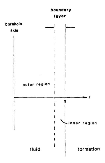
Figure 1: Boundary layer structure of the viscous fluid
