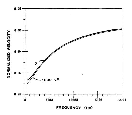
Figure 6: Stoneley wave phase velocity dispersion (normalized to the borehole fluid velocity) for viscosity values of 0, 1, 10, 100, and 1000 cP
