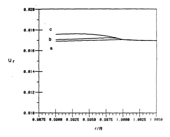
Figure 2: Stoneley wave radial displacement as a function of radial distance (normalized to the borehole radius) for viscosity values of (a) 1, (b) 100, and (c) 1000 cP
