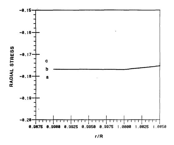
Figure 4: Stoneley wave radial stress as a function of radial distance (normalized to the borehole radius) for viscosity values of (a) 1, (b) 100, and (c) 1000 cP
