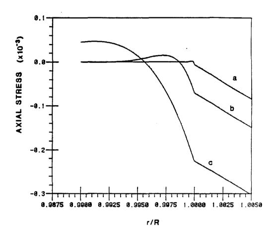
Figure 5: Stoneley wave axial stress as a function of radial distance (normalized to the borehole radius) for viscosity values of (a) 1, (b) 100, and (c) 1000 cP
