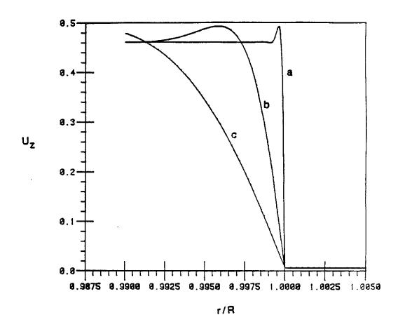
Figure 3: Stoneley wave axial displacement as a function of radial distance (normalized to the borehole radius) for viscosity values of (a) 1, (b) 100, and (c) 1000 cP
