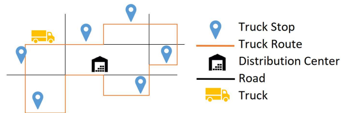
Figure 6. Truck-only Model. The Truck-only model is the conventional delivery where a truck delivers packages to customers from the DC.
