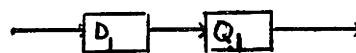
An Open Loop Quantizer System Used For The Test Upon The Input Signal of Q_1 (Figure 52)
