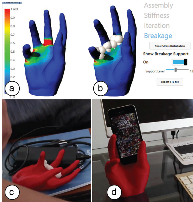
Figure 5. (a) Stress map, (b) breakage support. (c) Transporting the object, and (d) after dissolving the support material on arrival use the phone stand.
