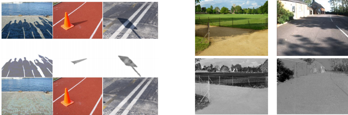
Figure 2-2: Shadow Removal. On the left: “Given an original image with a shadow mask (first row), the method is able to extract exact shadows (second row) and to automatically recover the shadow-less images (third row)” [21]. On the right: On the top images with shadows are shown and below the corresponding shadow invariant image [8].
