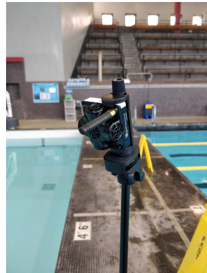
(b) Beacon System: units are mounted around the pool to help the Robot localize
