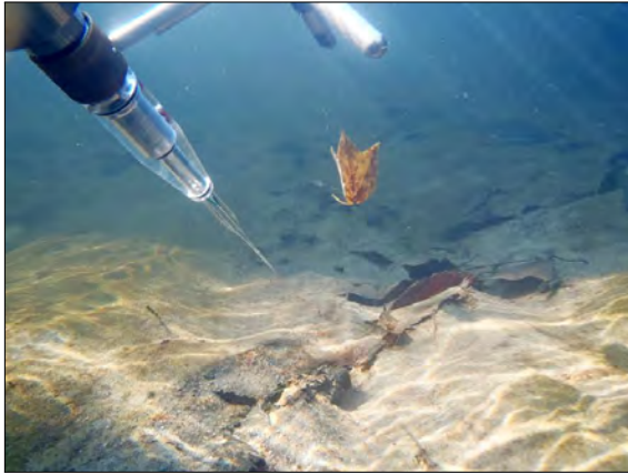
a) DO microelectrode mounted in EC system. Credit: Dirk Koopmans
