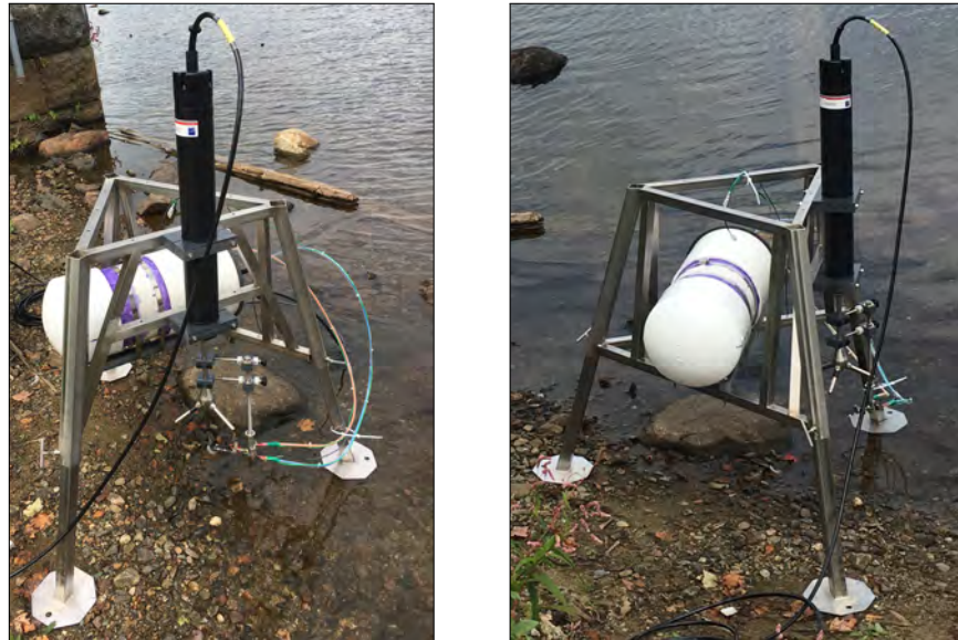
Figure 5.2: Benthic lander with all equipment assembled.
