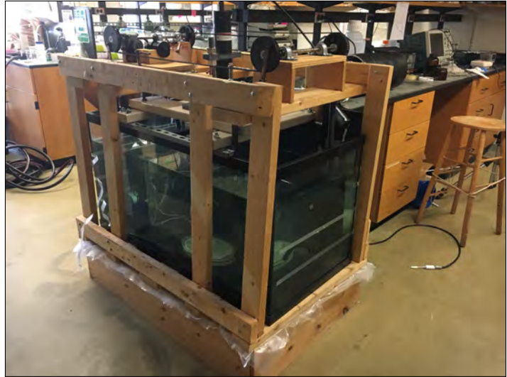
Figure 4.13: Experimental tank for conducting EC experiments. The wooden frame on which the tank rests holds a motor-driven mechanism with four oscillating plungers to generate turbulence.
