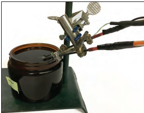
Figure 2.23: Experimental setup used for optical fiber calibration and spectral scan measurements. Use of a wide-mouthed 500 mL amber jar minimizes light leakage and LED reflections from glass walls, which can create a fat spectral tail for the LED signal that bleeds into the emission wavelength range.
