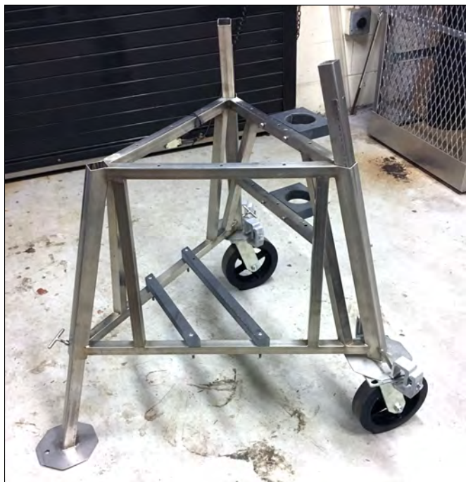
Figure 5.3: Benthic lander shown with clamp-on wheels for easier transport.
