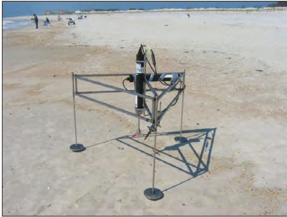
a) Lightweight EC lander used at many freshwater and marine sites. Credit: Peter Berg.
