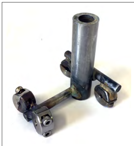
Figure 4.6: Holder for optical fibers, designed to reduce solid bulk while holding fibers at a 20 ° angle.
