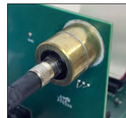
Figure 2.4: LED in lens tube
