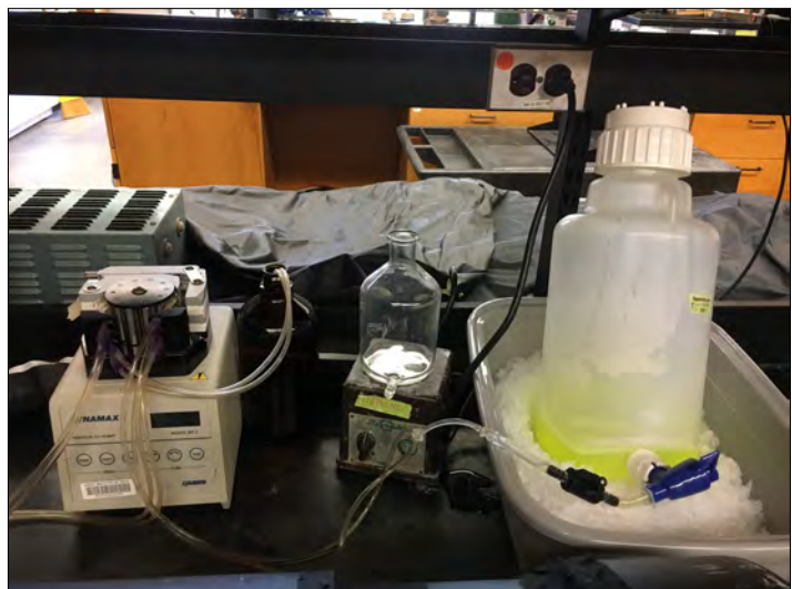
Figure 4.15: Benchtop setup of dye input system, including peristaltic pump with two channels for inflow and two channels for outflow. Inflow is connected to a carboy holding input dye, shown sitting in an ice bath. Outflow is directed to a separate bottle. The glass beaker with spigot used for inputting ambient tank water is also shown in the center.
