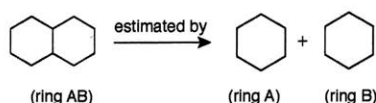
Figure 4.8: bicyclic AB correction estimated as sum of single ring A and B's corrections
