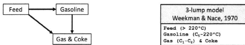
Figure 1.2: A simple lumped model for catalytic cracking process by Weekman and Nace. From Oliveira et al.
