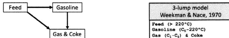
Figure 7.1: A simple lumped model for catalytic cracking process by Weekman and Nace. From Oliveira et al.
