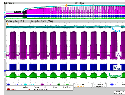
Fig. 26. Waveforms with 120V AC input and 12V DC output at 100W.
