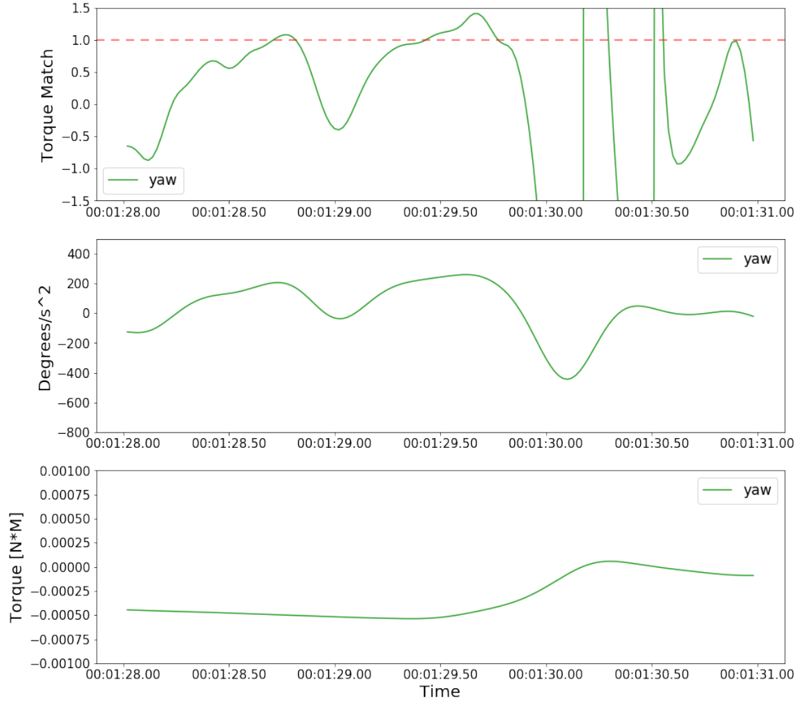
Figure 3-13: Yaw Torque Match \equiv I_{\hat{z}} * \alpha_{yaw} / (k_{motor} * \sum \pm RPS^2) . Vehicle torques itself in still air. There is a minor external interaction with a guide cord at 1m:29s. Match is not reliable as \sum \pm RPS^2 approaches zero.
