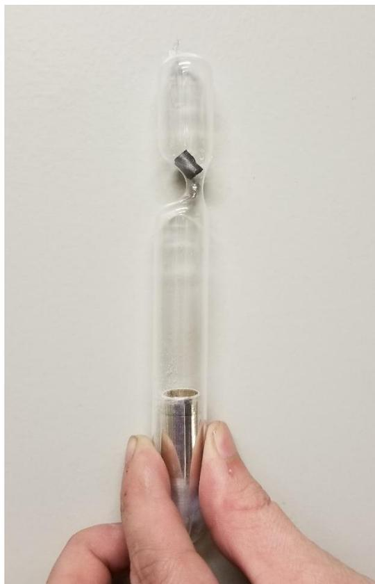
Figure 11. Image of silver crucible sealed with a piece of carbon in a quartz tube. In order to maintain that the getter remained above the crucible, the quartz was narrowed to form to compartments.
