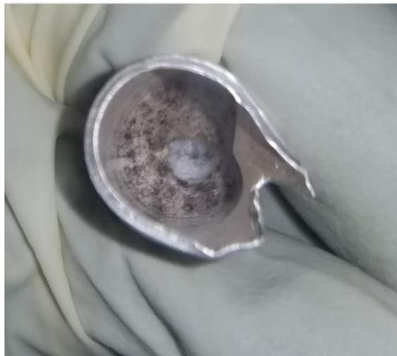
Figure 19. Image of second crystal grown at the PARADIM Bulk Crystal Growth Facilities. A hole can be seen in the center of the crystal. This reveals white crystal underneath, a sign of zone refinement.
