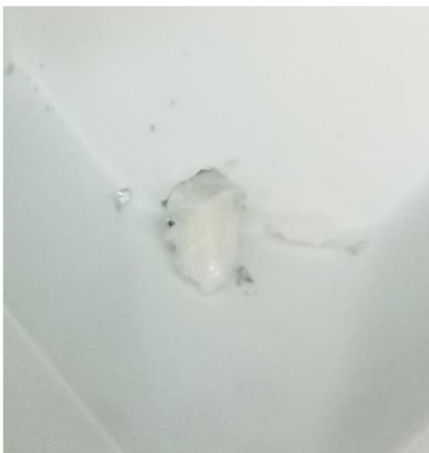
Figure 8. Photograph of the first slow cooling crystal. A small amount of aluminum foil is attached back of the crystal. Due to the rough shape of the aluminum foil crucible, the crystal was of an irregular shape.
