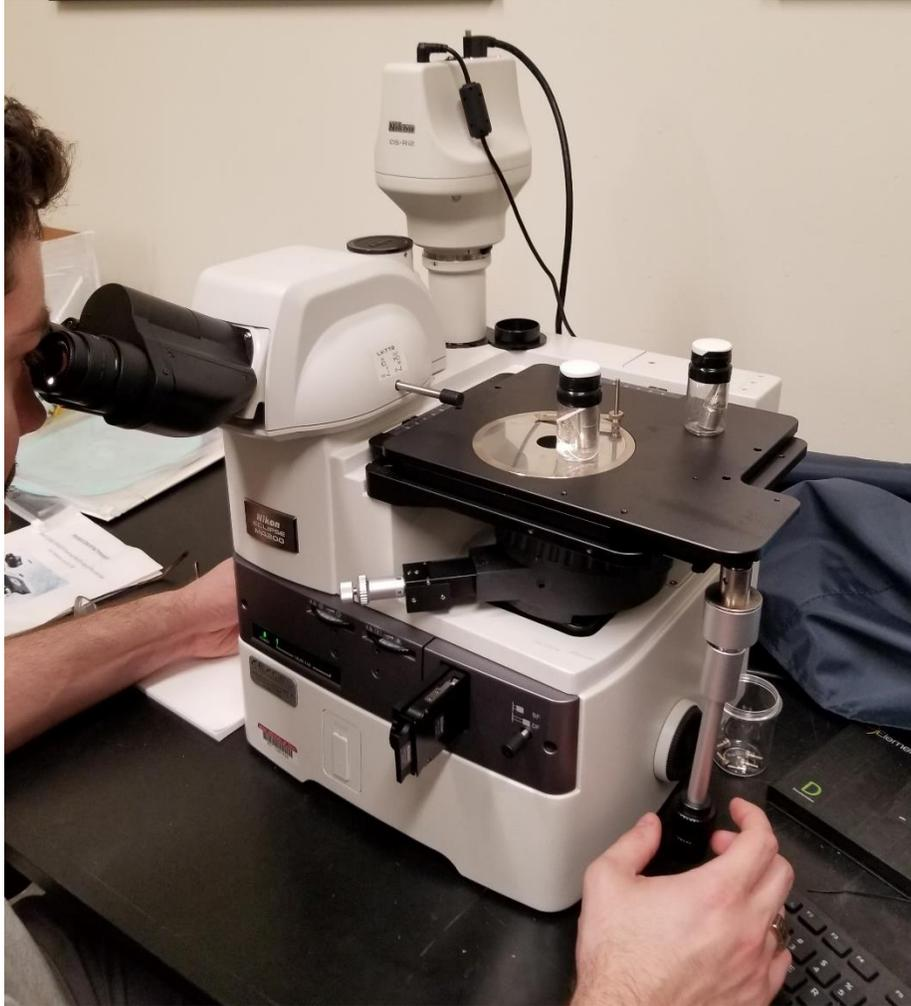
Figure 12. Due to the inverted configuration of this microscope, containment of samples within plastic vials was a simple and effective method for performing this method of characterization.
