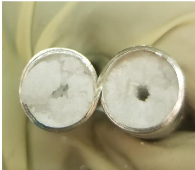
Figure 20. (Top) Image of surface of the third and final crystal that was grown at PARADIM. (Bottom) Cut cross section of crucible with crystal still encased.
