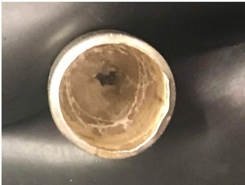
Figure 18. First attempt at crystal growth using PARADIM facilities. A gap ran down the center of crucible. The white scratches on the crystal near the crucible walls were due to collecting a sample to use XRD to confirm that sealing the crucible was sufficient to protect the charge material from moisture.
