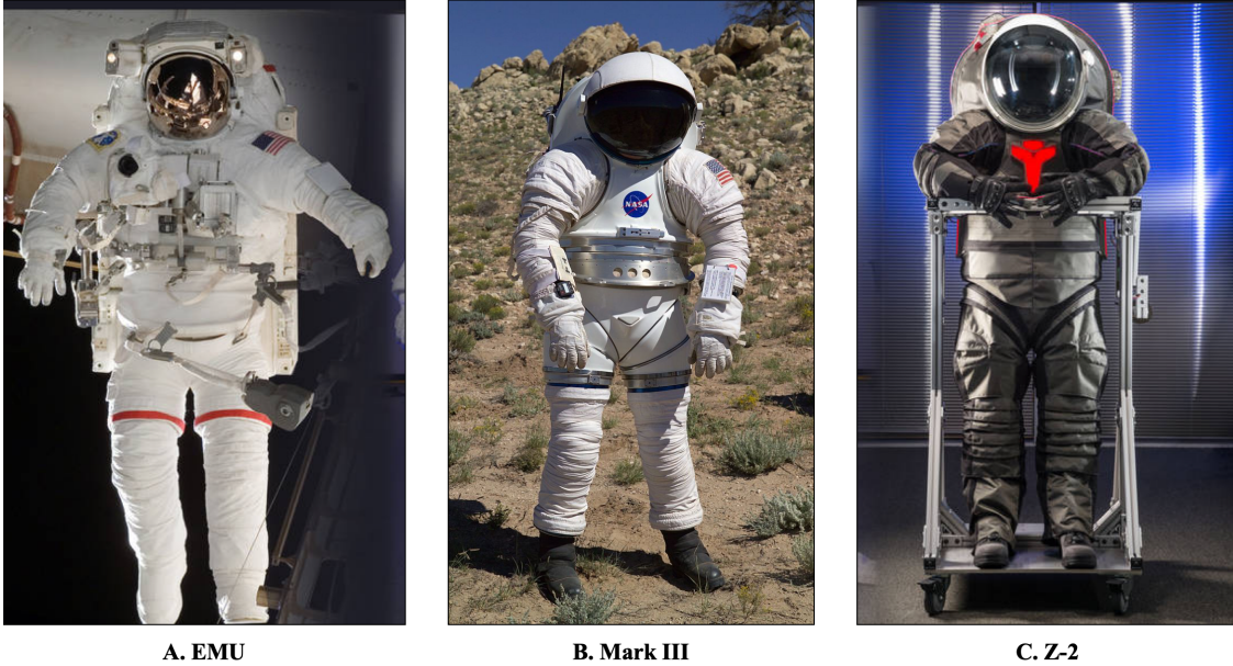
Figure 1.4: Existing Spacesuit Assembly Designs. A) The Extravehicular Mobility Unit (EMU) is designed for use in microgravity environment, while B) the Mark III is designed for planetary exploration. C) The Z-2 advanced suit concept is meant for use in both environments.
