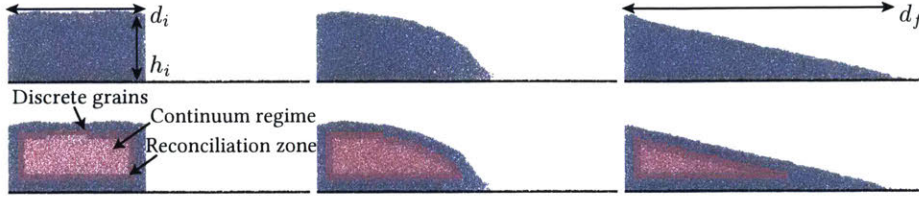
Figure 5-1: Granular column: A collapsing column simulated with DEM (top) and with our hybrid approach (bottom). Observe the nice agreement in the final profile with our hybrid approach and the purely DEM approach.
