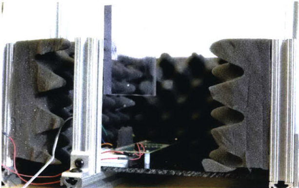
Fig. 11. Vertical gesture experimental setup.
