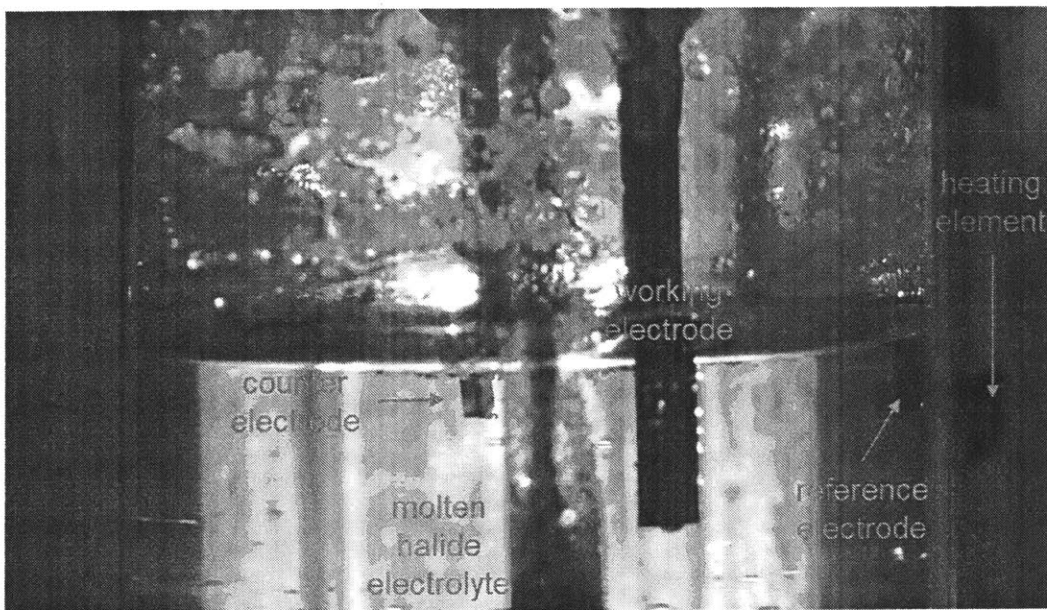
Figure 6-1: Electrochemical cell used in CER investigation. For dimensions, see text.
