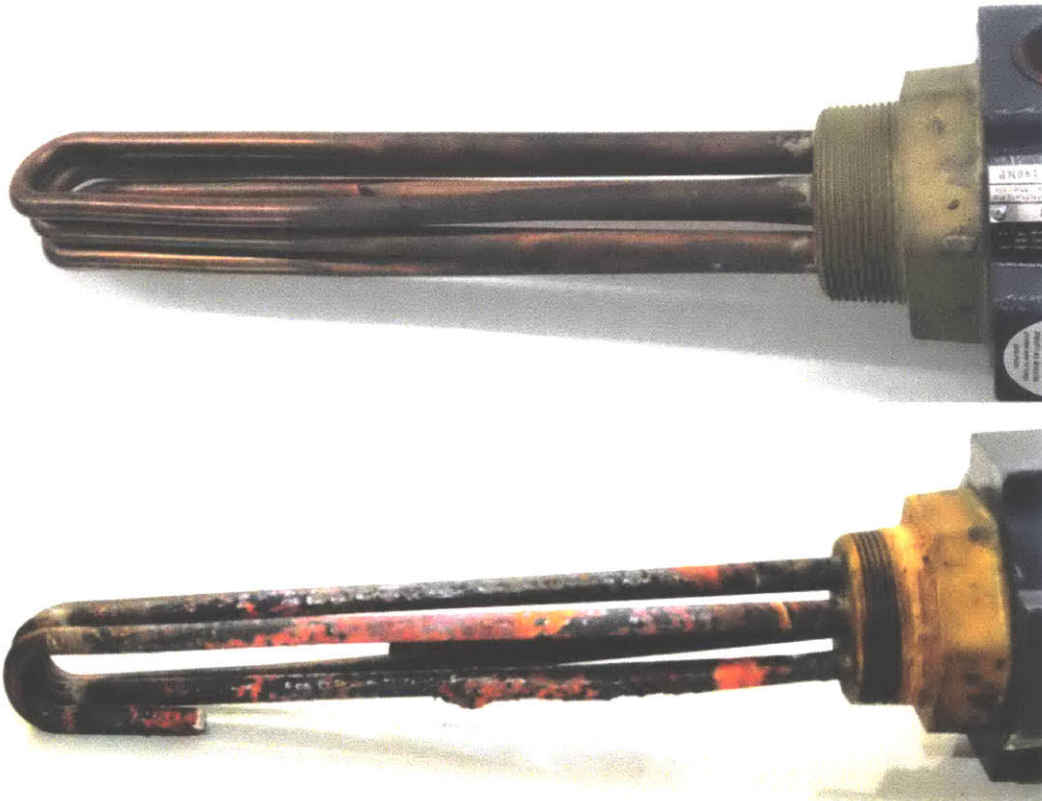
Figure 1-7: Top: New MPDE jacket water heater. Bottom: ESCANABA jacket water heater after removal.
