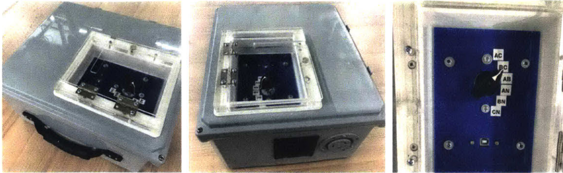
Figure A-2: External view of NC Calibrator. Switch (far right) allows for power to be safely shifted between line-to-line or line-to-neutral phases.
