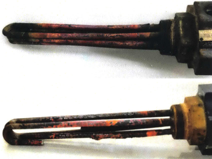
Figure 4-6: MPDE Jacket Water heaters removed from engines after electrical degradation was observed. Top: SPENCER port inboard heater, removed December 2018. Bottom: ESCANABA port Inboard heater, removed April 2019.
