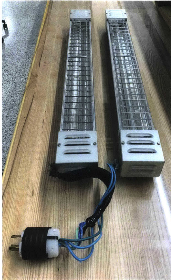
Figure A-5: Load used for shipboard non-contact calibration, consists of two 2500W heaters.
