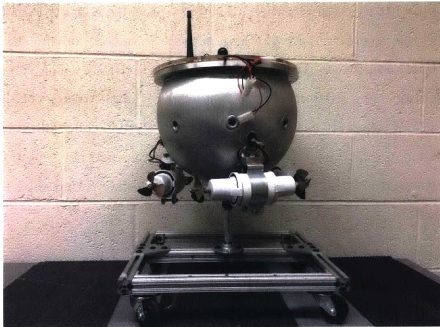
Figure 5-2: Modified buoy for sub-surface operation.
