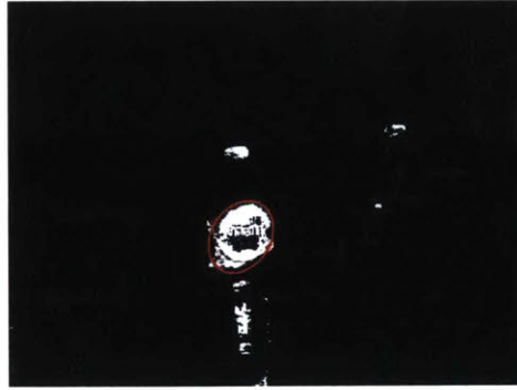
Figure 3-3: Sample of a probability distribution generated by histogram back-projection.
