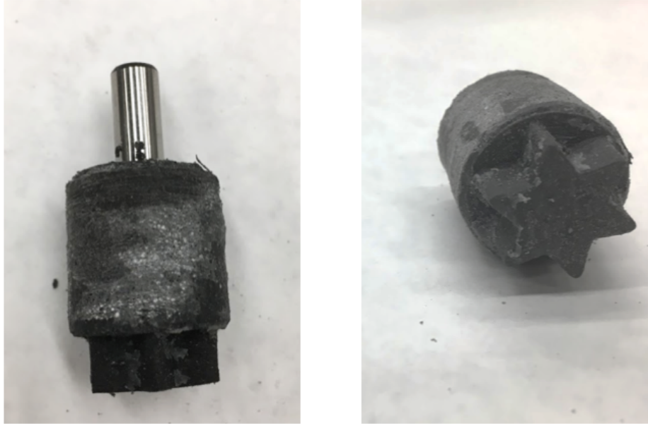
Figure 3-6: The starter pocket tool molds a star-shaped pocket into the aft end of the propellant grain. This creates more propellant surface area for ignition and provides a mounting location for the starter propellant grain.
