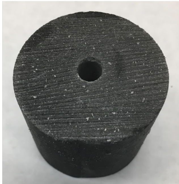
Figure 4-4: Propellant samples were drilled with 1/4" holes for mounting to the sliding sample mount. Note: This image was taken after the peel tests, so the liner has already been removed.
