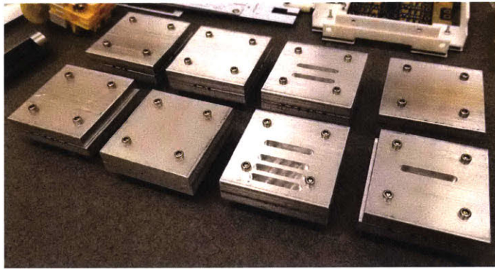
Figure 3-4: Different lids tested for better quenching.
