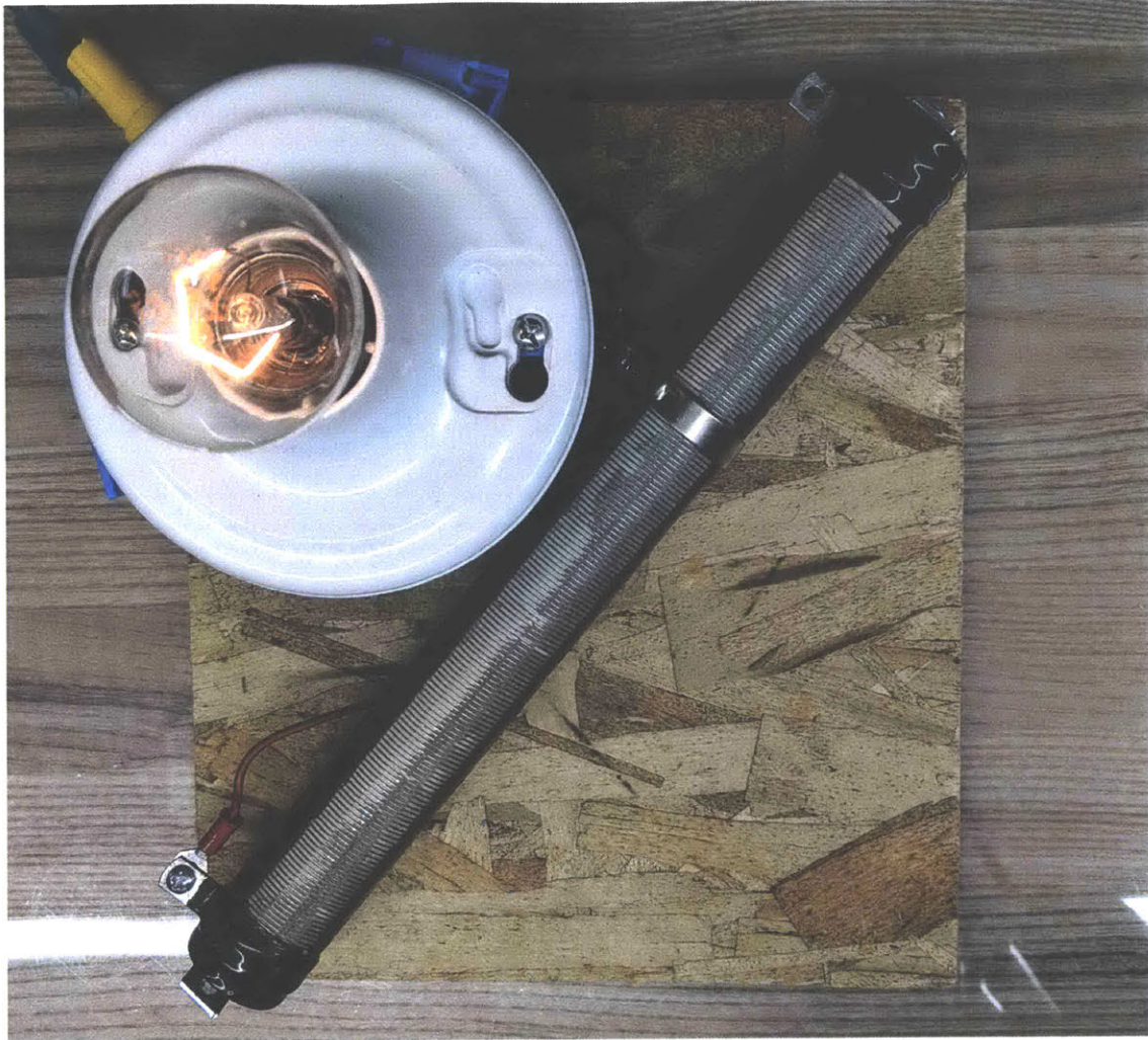
Figure D-3. A photograph of the load connected to the model-scale system.
