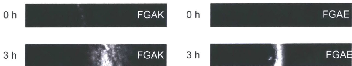
Figure 4.S5 Verification of hydrophobic domain availability in FG peptide gels. Transport of Nile Red into FGAK and FGAE gels after 0 h and 3 h of incubation. Fluorescence indicates that the dye is able to access hydrophobic environments created by FG domains within the gels. Images are of representative gels from three independent replicates.
