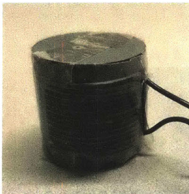
Figure 2-11: Prototype inductor of the example design (Section 2.4) having a measured Q of 720. Vertical windows in the outer shell were added to impede the circumferential component of flux and to allow the winding terminations to leave the structure.
