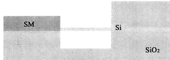
Figure 5.1: Fully oxide-clad waveguide with shape-memory phase shifter.
