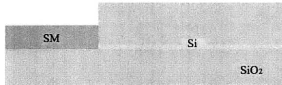
Figure 5.1: Fully oxide-clad waveguide with shape-memory phase shifter.
