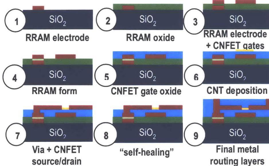
Figure 3.3: Fabrication process flow of SHARC.
