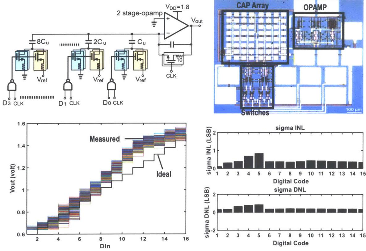
Figure 3.5: 4-bit capacitive DAC with SHARC. (top) Schematic and die photo. (bottom) Measured characteristics show the monotonic behavior with offset (50mV) and non-linearity where the maximum  $\sigma_{INL}$  and  $\sigma_{DNL}$  is 0.8 LSB.
