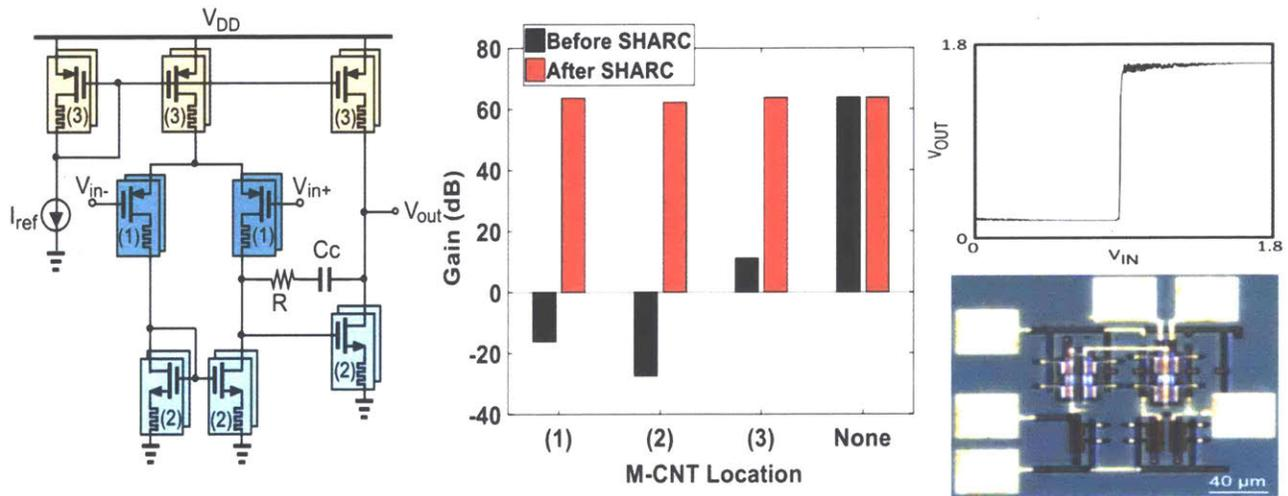
Figure 3.4: Two-stage op-amp with SHARC. (left) Schematic. (middle) Gain (dB) of op-amp when an m-CNT is located in different locations of the op-amp (labeled in schematic) before and after SHARC. Before SHARC, gain can reduce by >100 dB, while after SHARC gain is reduced by a maximum of 3 dB. (right) Die photo and experimental measurement of op-amp using SHARC, achieving gain >800.
