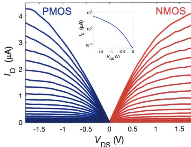
Figure 2.3: Characteristics of PMOS and NMOS CNFETs with a channel length of  $\sim 2.5\text{ }\mu\text{m}$  and width of  $\sim 4\text{ }\mu\text{m}$ .  $I_D$ - $V_{DS}$  curves show well-matched CNFET CMOS (i.e., with similar on-current for both NMOS and PMOS).  $V_{GS}$  range from 0 V to  $V_{DD}$  (1.8 V) with an increment of 0.1 V (for NMOS,  $V_{GS}$  from 0 to  $-V_{DD}$  for PMOS). Inset shows an  $I_D$ - $V_{GS}$  curve of a PMOS CNFET with  $I_{ON}/I_{OFF} > 8000$ .
