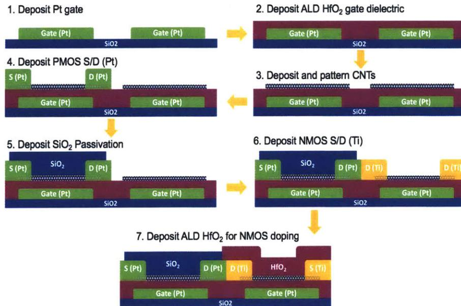
Figure 2.2: CNFET CMOS process flow. A back-gate geometry is used for both the PMOS and NMOS CNFETs. All low-temperature ( $<250^\circ\text{C}$ ) processing is performed with solid-state and silicon CMOS compatible materials.
