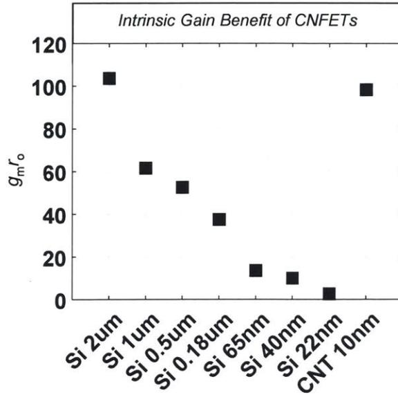
Figure 2.1: Intrinsic gain ( $g_m r_o$ ) [Razavi 2017] benefits of CNFETs. The intrinsic gain is extracted from circuit simulations (Cadence Spectre®) using commercial process design kits (PDKs) for silicon CMOS and using an experimentally calibrated compact model for CNFETs (calibrated using CNFETs with sub-10 nm channel length) [Lee 2015].
