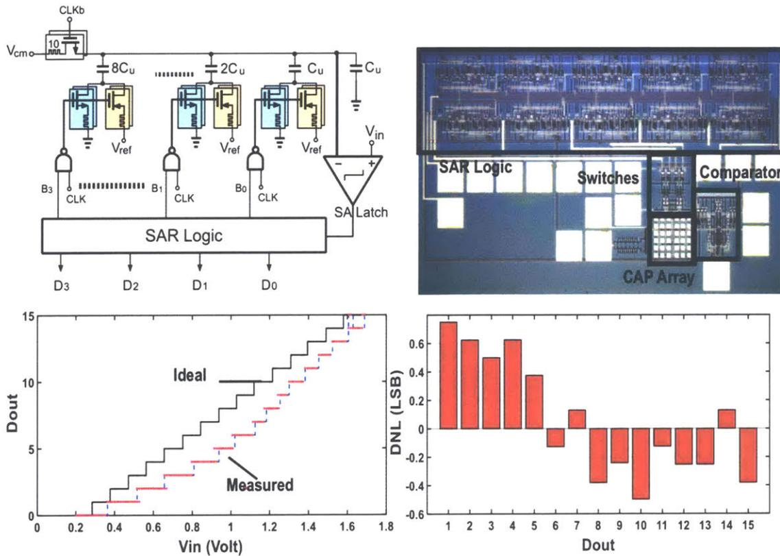
Figure 3.6: 4-Bit SAR ADC with SHARC. (top) Schematic and die photo. (bottom) Measured characteristics show the ADC behavior with offset (35mV), non-linearity and gain error whereas the DNL (-0.5 LSB $\rightarrow$ 0.75 LSB).
