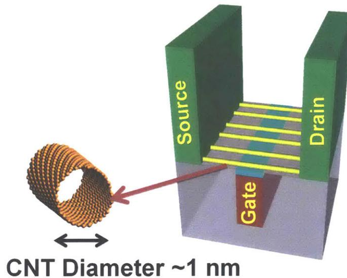
Figure 1.1: Schematic of carbon nanotube field-effect transistor (CNFET) with multiple parallel CNTs (nanocylinders made with atomically thin sheet of carbon atoms with diameter  $\sim 1$  nm) bridging the source to drain contact. Conductance of the CNTs are modulated by the gate to turn the transistor on or off.
