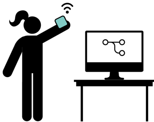
Figure 1: Concept of the presented design toolkit. A wearable or smart device with (potentially attachable) sensors can be reconfigured wirelessly by using a graphical web application.
