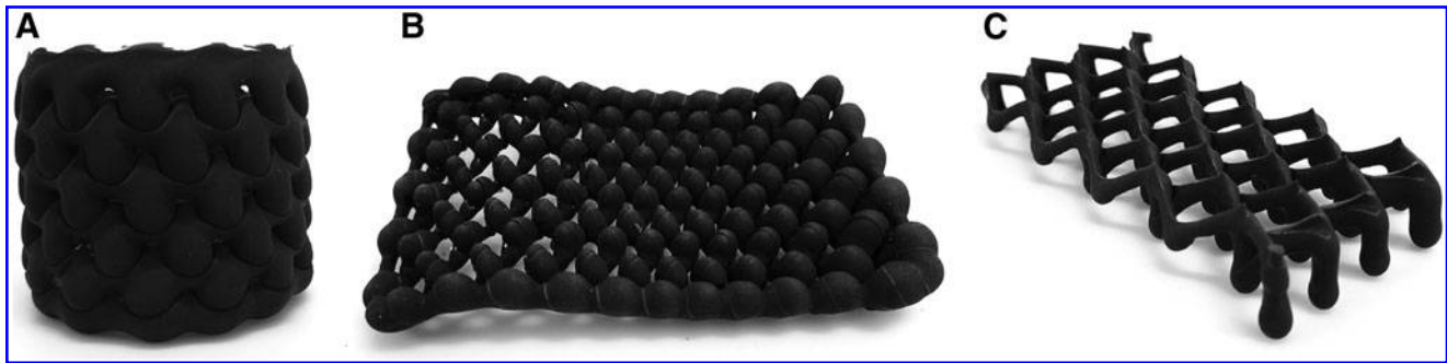
FIG. 5. (A–C) Polyurethane rubber printed parts with various shapes and connections. (A) Ball-joint cylinder. (B) Variable surface. (C) 2.5D Lattice.
