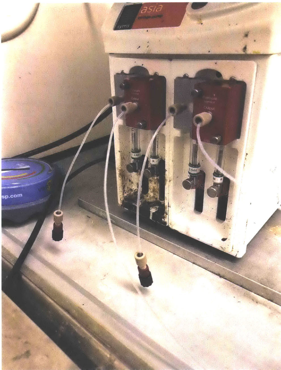
Figure SI- 2. Closer examination of Syrris Asia syringe pump with tubing connected. Shown are a pair of “dual” pumps, i.e., one pump refills from a source while the other pumps solution out.
