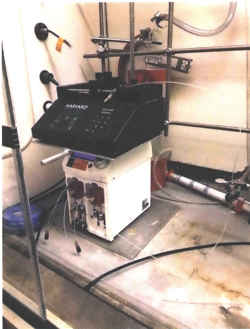
Figure SI- 1. (top) Harvard Apparatus PHD 2000 Infusion syringe pump. (bottom) Syrris Asia Syringe Pump. Both were used in the continuous-process for benzyne generation.
