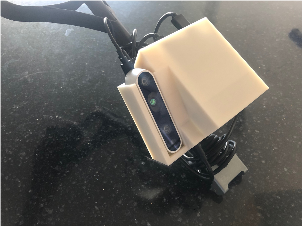
Figure 3-1: The whole device with components connected, placed in the case, and mounted on the guide dog harness handle.
