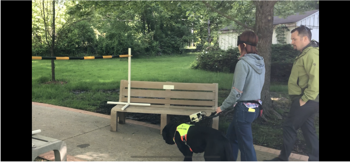
Figure 5-1: Blind-folded test subject approaching an obstacle with device mounted on guide dog harness
