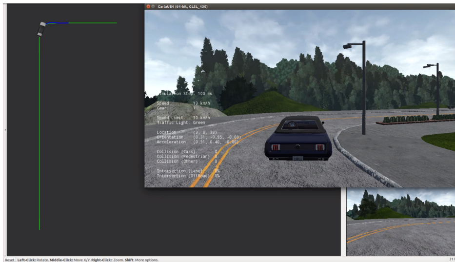
Figure 3-9: RViz visualization of the CARLA vehicle following the challenge path. Reference path is shown in green, and pure pursuit goal path is shown in blue. Also shown are the a third-person view of the CARLA vehicle (upper right) and a first-person simulated camera view from the front of the vehicle (lower right).
