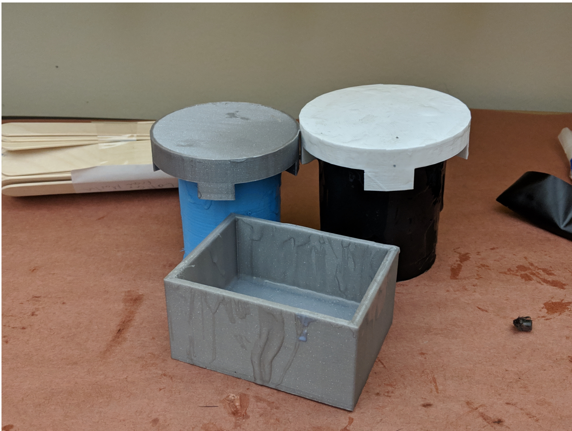
Figure 14. Examples of molds used for fabrication. A single rectangular mold is sufficient for fabricating a flat CurveBoard, but the cylindrical cup requires the two sets of two molds in the back. Additionally, the blue mold needed to be printed in TPU, a flexible material, in order to extract the cured product.
