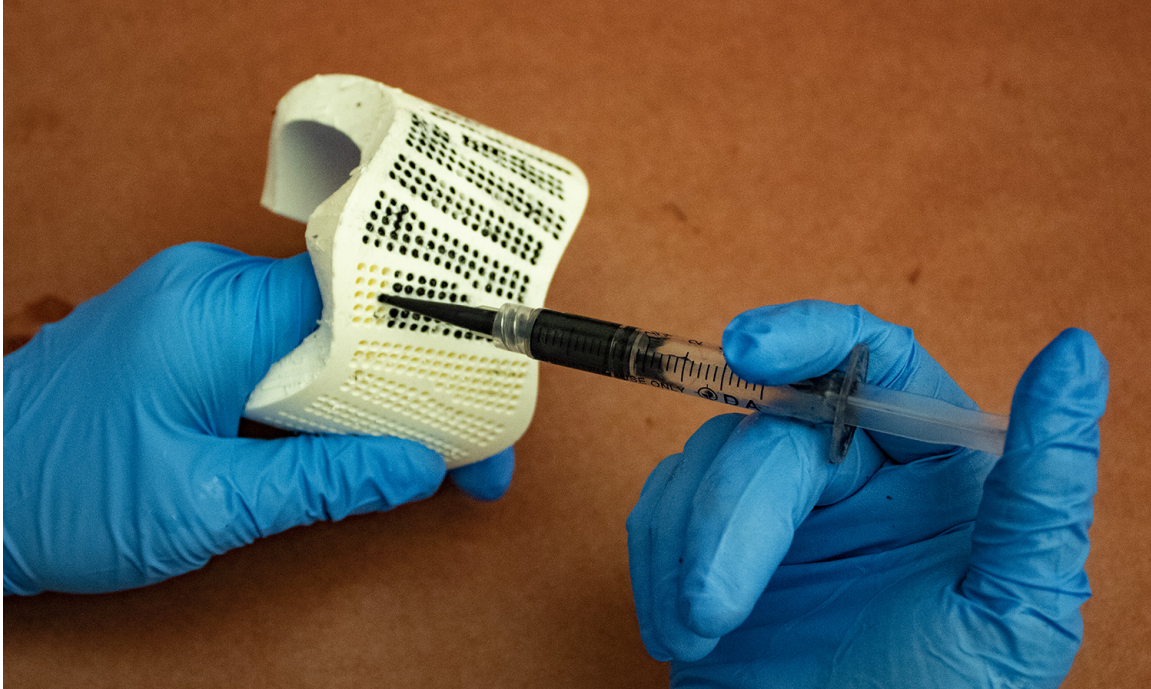
Figure 7. Filling the hollow channels of the CurveBoard with conductive silicone.
