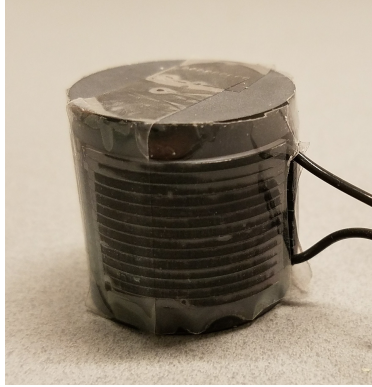
Figure 3.2: Prototype inductor of the example design (Section 3.1) having a measured Q of 720. Vertical windows in the outer shell were added to impede the circumferential component of flux and to allow the winding terminations to leave the structure.
